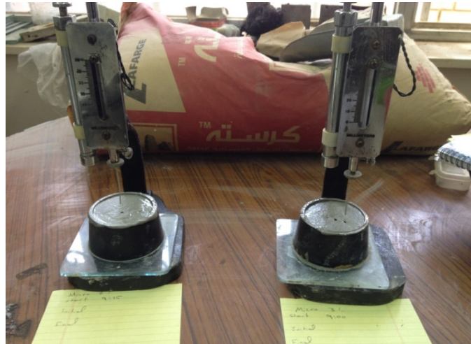
Figure 3.9 - Setting time test by using vicat apparatus
